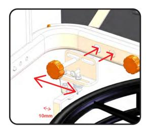
Now fit the brake assemblies using the supplied M8 screw and washer. Before tightening be sure to set the brake up properly.
