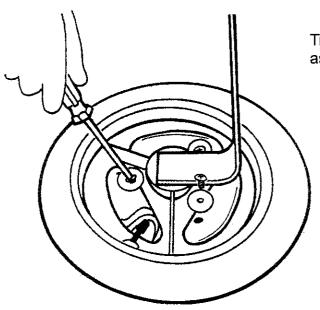
Tighten the three Phillips head screws as shown to secure hub to wheel.
