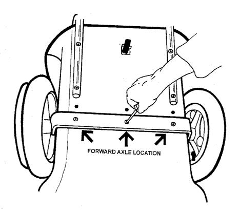
The Ready Racer axle can be positioned in the forward axle location to allow smaller children or children with limited arm range of motion the ability to move the wheels easier.
