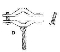
Remove one screw from one clamp. (See illustration D.) This clamp and screw will be used in step 7.
