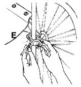
6. Place one clamp on either the left or right side of the wheelchair frame approximately three inches below the seat, (See illustration E.) Tighten screws enough so that clamp stays in place, but not so tight as to prevent clamp
