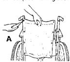
2. Remove existing backrest. This is done by removing the eight screws that secure the backrest to the wheelchair frame. Do not discard screws. Two of them will be needed to install Reclining Backrest. (See Illustration A.)
