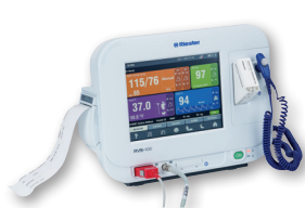
Integrated thermal printer (optional)
