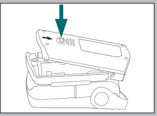
**STEP 1.** Install two AAA batteries into the battery cassette, and press the button down along the arrow and push the battery cover. Then close its cover.
