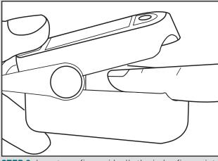
**STEP 3.** Insert one finger, ideally the index finger, into the opening of the pulse oximeter, please ensure that the patient's nail is facing upwards.
