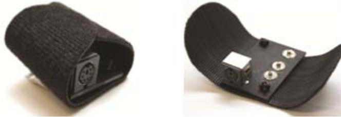
This adapter allows EMG A to accept the intracavity sensors or external pelvic muscle electrode lead wire sets for incontinence applications. Open the Velcro sleeve, match the female snaps on the end of the Pathway™ Preamplifier (part# 2583) cable with the male snaps of the Pathway™ Adapter (part# 3660), connect and re-wrap the Velcro sleeve. Note the six pin mini din connector input at the end of the Pathway™ Adapter (part# 3660).
