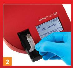
Insert microcuvette into analyzer.
