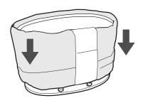
Remove the paper band and pull up OUTER LAYER of refill and push it down through the middle of the cartridges.
