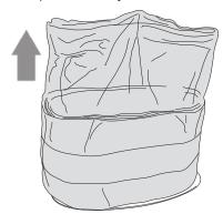
4 Pull refill liner down through the middle of the cartridge.
