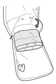
Pull refill down through the middle of cartridges and tie a knot.
