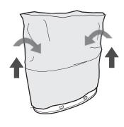
Re-attach the cartridges, with the newly installed refill.
