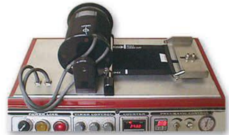
Cuff hook and loop adhesive test
