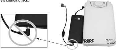
2. Plug the external battery discharge cable into the power jack on the EasyPulse POC.
