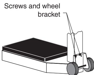
Use the two 10-32 x 3/8 self-tapping pan-head screws in the back of the column to attach the wheel bracket.
