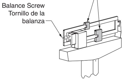
To balance scale, move both poises to zero (0) and turn balance screw to right or left until scale balances. For accurate weighing, place scale on level floor.
