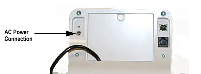
Figure 2-5. Power Connection Site
