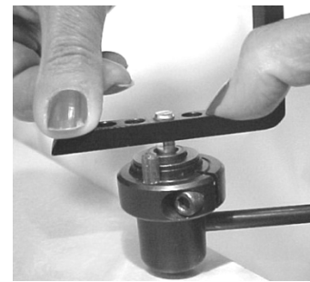
Reattaching L-bar with Down Stop in front.
