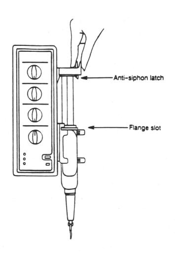
WARNING: ASSURE THE SYRINGE BARREL FLANGE IS PROPERLY INSERTED INTO THE HOLDER'S NOTCH OR UNCONTROLLED EMPTYING MAY OCCUR.
