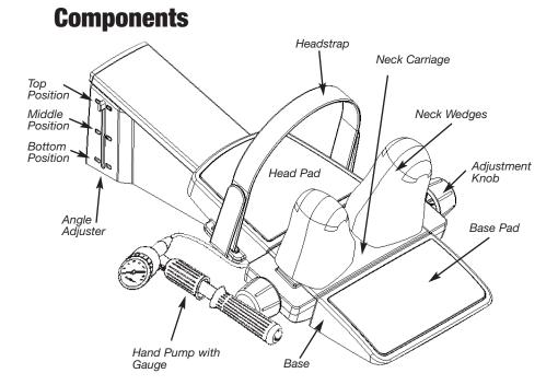
Figure 1. Components of the Saunders Cervical Traction device.
