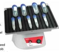
without tools or disassembly; simply grip the platform and move to the desired angle. Low speeds and a minimal tilt angle create a gentle wave motion, required for most blot washing. Higher speeds and steeper angles produce more aggressive agitation for vigorous sample mixing. Rotator comes standard with autoclavable dimpled and flat mats and maintenance-free, brushless motors.
