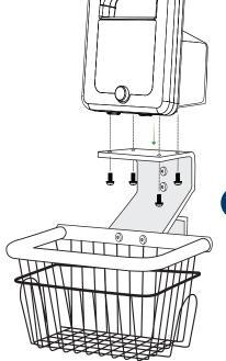
Align holes on bottom of the ADView 2 with the four holes on the mounting bracket as shown.
