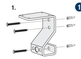
Attach wall bracket to wall before assembling basket. For optimum viewing, it is suggested that you measure 60" from the floor to the top of the wall mounting bracket (or adjust as needed). Once positioned to desired height, mark screw positions on the wall making sure bracket is level. Screw in the three supplied screws (5600-HW-01) firmly into a stud, or use the three supplied mollies and secure to the wall.
