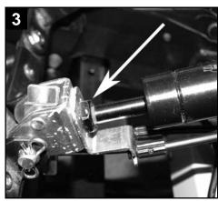
4. Remove the opposite end of gas spring by removing the cotter & clevis pin.
