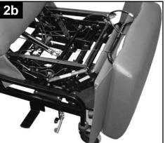
3. Locate the gas spring and loosen the nut on the gas spring using an 11/16" wrench.
