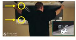
**NOTE:** The Snap Switch which is located in one of the top right hand corner of the UV Chamber, will be deactivated when the UV Chamber lid is removed.
