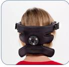
The mounting disk accommodates a I" (25mm) ball. The disk can be removed to attach custom hardware using M5 screws.
