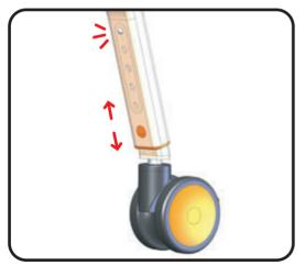
To adjust the Seat Height adjust the Caster Legs (part #500-296 front & 500-010 rear) by using the Push Pins in the legs and ensure that the push pins fully engage the height adjustment holes evenly.
