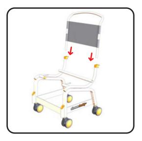
Slide Back Rest Frame (part #500-372 for 22 and 377 for 26) down through Arm Clips (part #500-237) and into the Seat Frame (part #500-021). Make sure that push pins are fully depressed before inserting the back rest frame.
