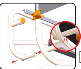
To fully remove an arm rest from the chair, depress the push pin (part #500-269) fully allowing the arm rest to be pulled outwards from the seat frame tube. To re-fit the arm, reverse this action.
