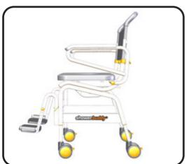
The chair may be adjusted to have a higher seat height at the front and lower at the back to suit user requirements. This can be accommodated by adjusting the front caster leg only to be extended further than the rear caster leg. Under no circumstances should there be more than 1-adjustment position difference between front and rear (approximately 20mm).
