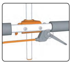
Check to ensure that when the handle is squeezed in then released that the handle springs back into the position shown.
