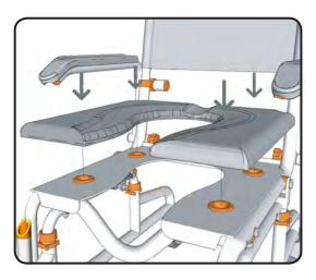
Ensuring the correct orientation attach the seat cushion to the seat base by pushing the 4 locating lugs on the underside of the cushion into the connectors on the seat base.
