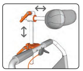
Before using the chair adjust the neck rest so that it provides the correct support for the intended user. Unscrew the neck rest handles to allow the tubes to easily slide for adjustment.
