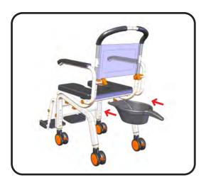
The Commode Bucket (part #500-072) can be pushed into position from the rear of the chair and is held in position by the Commode Bucket Connectors (part #500-095) pre-fitted to the cushion at the factory.
