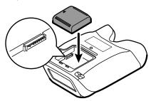
For battery replacement, remove the existing battery and then insert the new replacement battery into the battery compartment.
