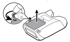
3. For first-time setup of the RetinaVue 700 Imager, insert the battery into the battery compartment.
