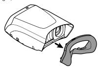
attach the Anterior Imaging Spacer to the RetinaVue 700 Imager, and then attach the face cup to the Anterior Imaging Spacer.
