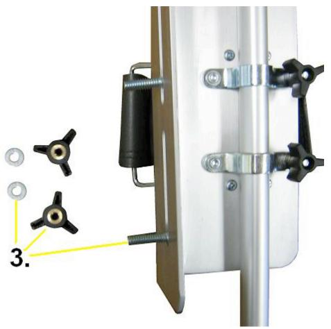
4. Put the two carriage bolts into the platform crutch bracket as shown.
