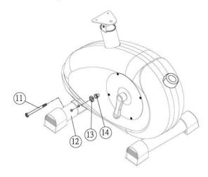
1. Attach the rear support tube (No. 12) to the frame using the Allen key and bolt M8\*65 (No. 11).
