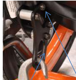
Rear Securement with wheelchair anchored seat belt anchor
