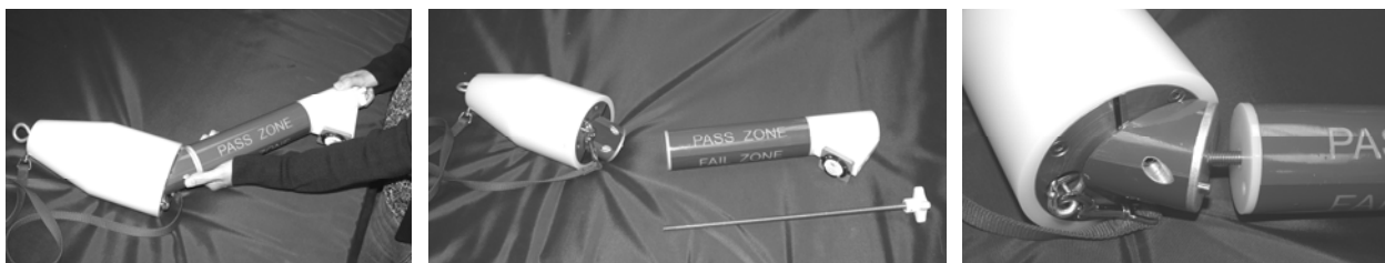
Figure 6. Disassembly and assembly of the cone and cylinder tool.
