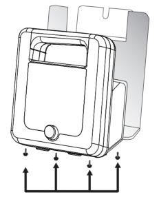
Once fully seated, use the hex key to screw in the four mounting screws through the bottom of the caddy into the ADView 2. Hand-tighten all four screws until firmly set.
