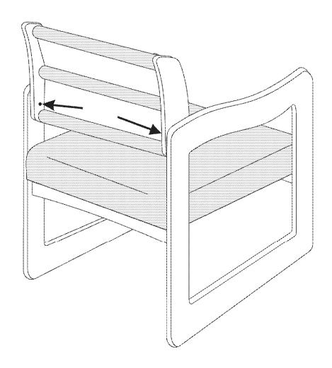
To prevent tampering, an optional locking screw has been provided. Once chair is completely assembled, make sure that the back is slid completely into brackets of side frames. Place screws that are provided into holes in the back side of the back rest being sure that the screw lines up with the small hole on the side frame. Screw in until the screw is snug. Cover with "snap-cap" provided. Repeat with other side.
