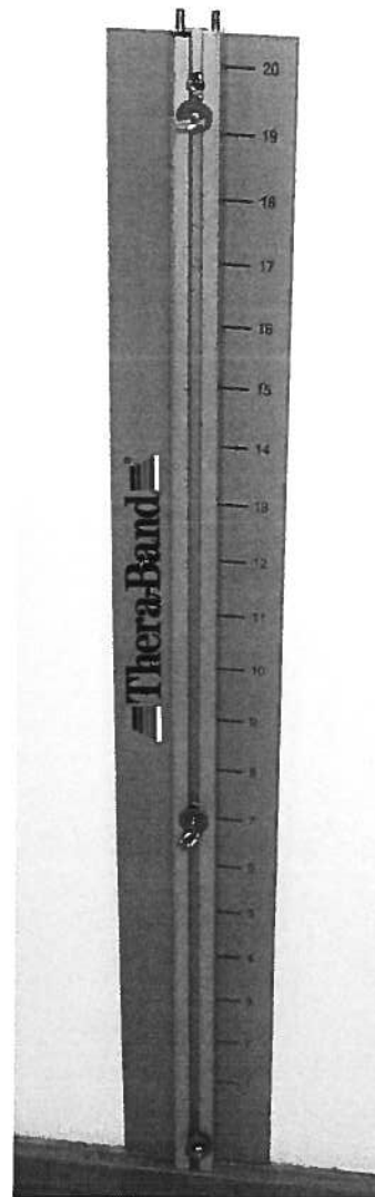
Figure 1 – Lower track (two eyebolts) mounted on wall near floor (lower hole has washer under screw-head).
