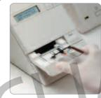
Immediately place the cassette into the Analyzer drawer with the black reaction bar toward the Analyzer and the brown magnetic stripe on the right.
