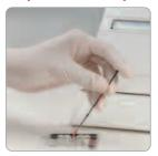
Place the end of the capillary tube into the sample well and dispense the sample by pushing down on the plunger. Keep the cassette level after the sample has been applied.
