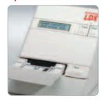
Press the **RUN** button on the Analyzer. The cassette drawer will open, and the screen will display: Load cassette and press RUN.
