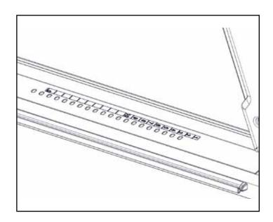
To move the seat assembly push down on either left or right side yellow foot levers and hold, then push the seat assembly forward or backward to the desired position along the adjustment pan.
