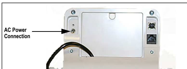
Figure 2-5. Power Connection Site
