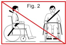
Do not allow belt restraints to wrap around or over wheelchair components as this will keep them from fitting securely across the body.
