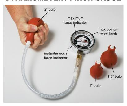
Adjustable dynamometer/pinch gauge measures both grip and pinch strength. Comes with three different sized interchangeable squeeze bulbs that can be easily fitted to the gauge. Lightweight and portable. Maximum reading remains until reset by turning center knob. Unit is calibrated in PSI (0-30) and kPa (0-200).
