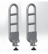
2. Clamp the rail bracket over the edge of the bed deck with the vertical sliding steel plate positioned on the inside of the bed frame. Tighten the two Allen screws and rotate the turn knob underneath the bracket clockwise until the rail is secured in place. Repeat the procedure to install the bed rail on the other side.
