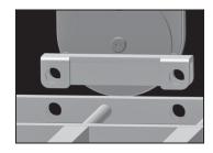
Re-insert the metal pins through the mounting holes and secure with the snap rings. Make sure the snap rings are positioned in the groove of the metal pins. Repeat the same procedure to install the other rail.
